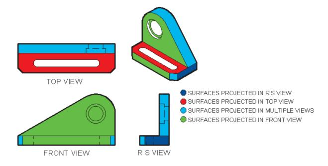
take time and try to visualize the views of the 3D object as they are projected into the top, front , and right side view.
