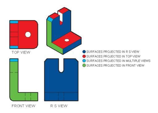
take time and try to visualize the views of the 3D object as they are projected into the top, front, and right side view.
