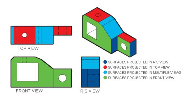
take time and try to visualize the views of the 3D object as they are projected into the top, front , and right side view.
